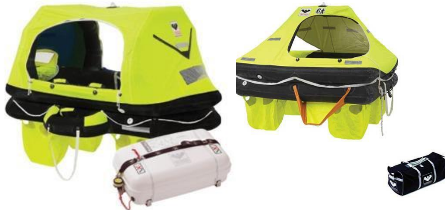
Offshore raft in hard container (Viking) and Coastal raft in valise pack (Viking)
