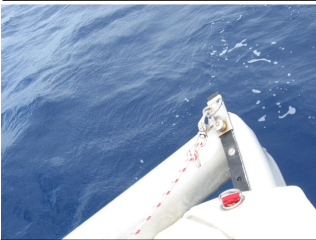
4 – Too much load on the spinnaker pole, as evidenced from the ring.
