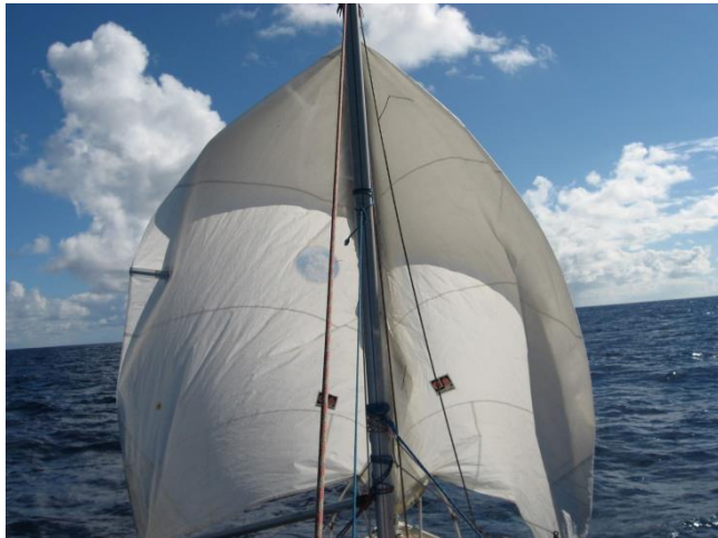
11 – Phase III of jury rig! Top portion of mast is up and headsails are flying! This rig was stable and took me to the finish line.
