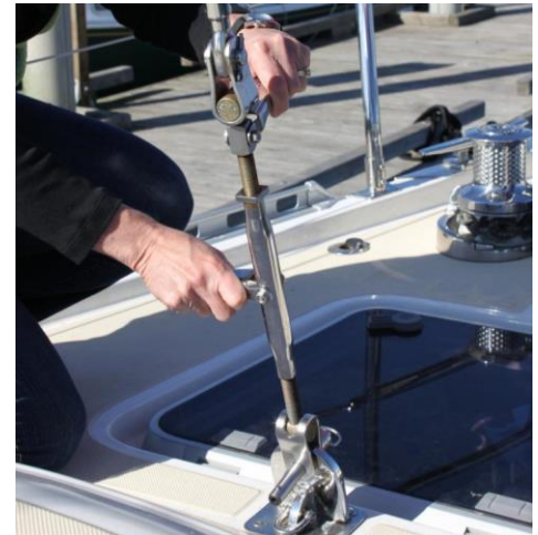
Hand-adjustable turnbuckle allows removable stay to be tensioned, note removable pin at base, Carol Hasse photo
