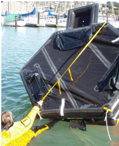
Righting a raft from water, SLH photo
