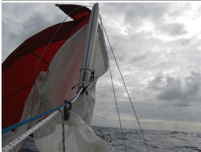
7 – This was early evening on the day of the dismasting. I put up the bottom portion of the mast to keep the boat stabilized. Not pretty but it worked.
