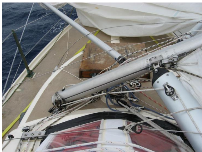
1 – Mast is disengaged from the step. A few scratches, but no harm done to the deck.
