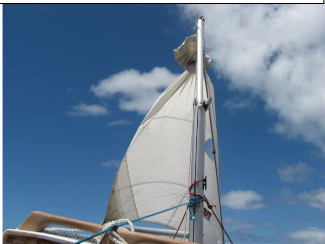
9 – Phase II of the jury rig. I opened up the mast and stuck the bent spinnaker pole in. Again, not pretty but it kept me going in the right direction.
