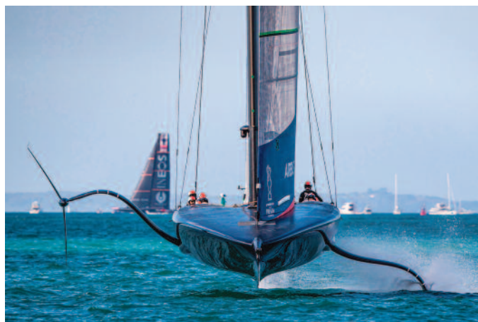
The standard-issue foils used in the 36th America's Cup did not always operate as expected on the AC75s.
